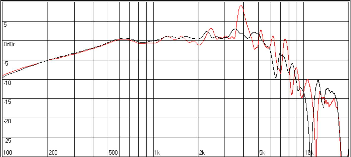
Figures fifteen and sixteen show the stock impulse and frequency response for a typical paper cone body 5.25-inch transducer. The upper limit of its bandwidth is defined by a prominent diaphragm material vibration mode (cone breakup). In this application, the vibration modes for the dust cap are well into the transducer's stop band and are not critical.
