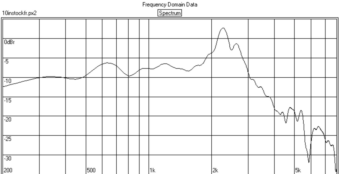
The performance change after application of targeted impedance changing techniques is shown in the two graph below on this page. The frequency response graph of the modified cone and dust cap also has the stock frequency response graph drawn on top in red for easy comparison.
