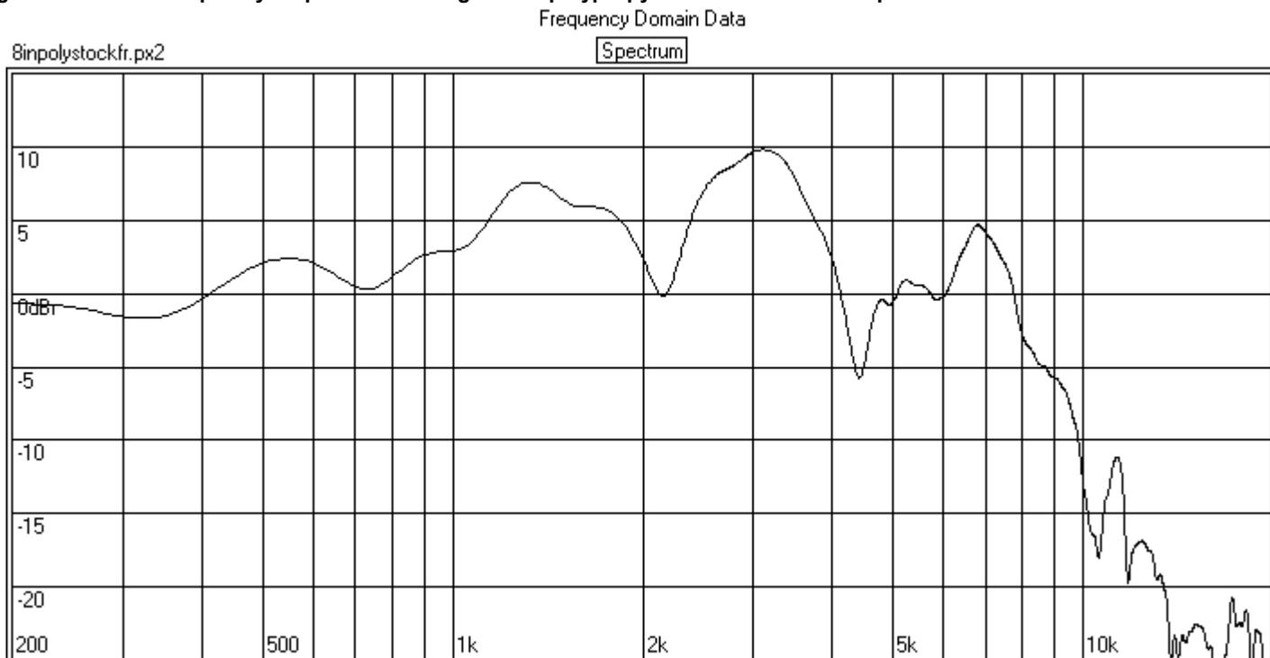
One technique for simplifying vibration mode problems in transducers is to replace the dust cap with a plug (sometimes called a phase plug) where the application will allow. Figures seven and eight show the eight-inch polypropylene coned transducer with the dust cap replaced with a plug.
