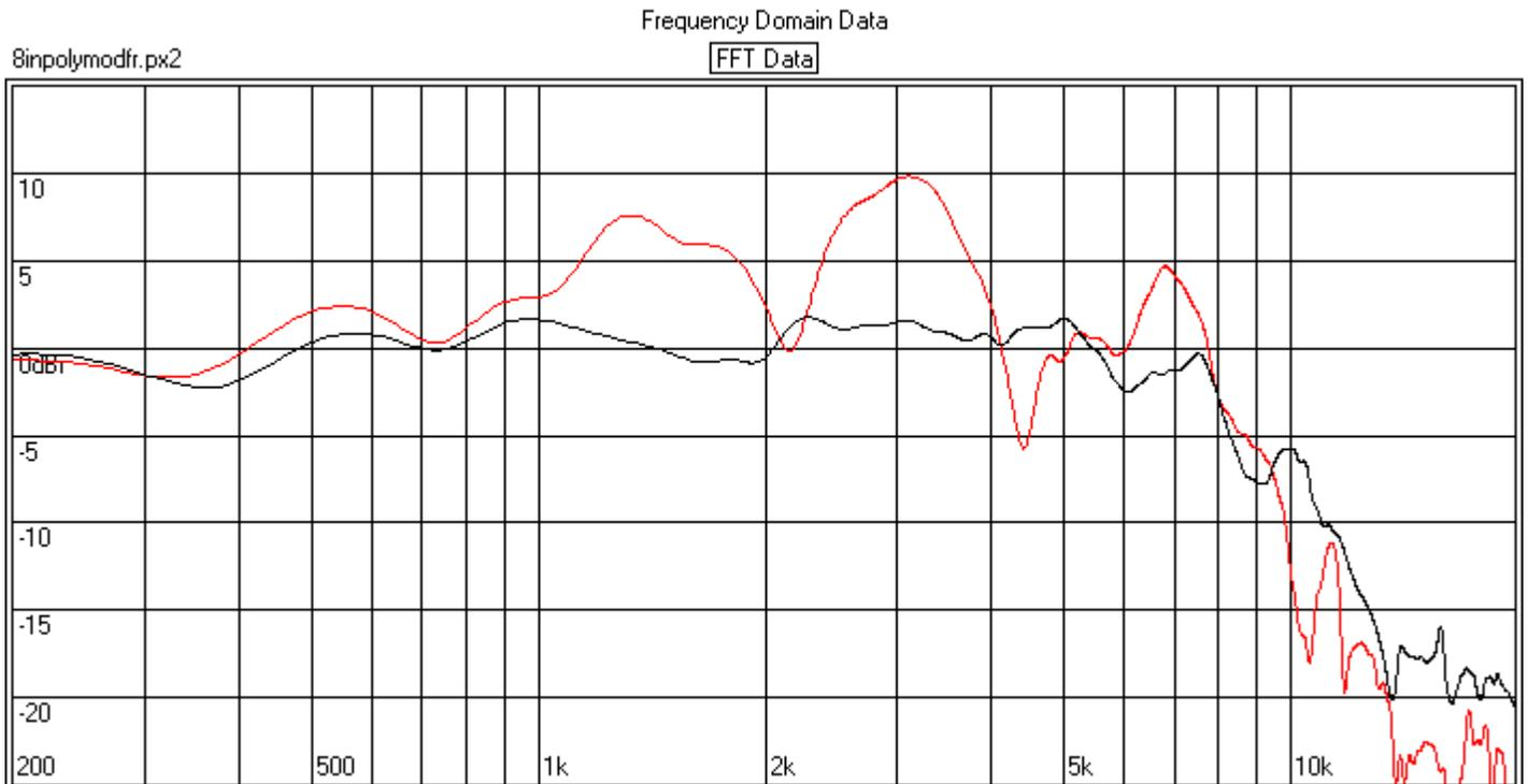
Figures eleven and twelve show the stock impulse and frequency response of a second eight-inch advertised basket diameter transducer. This transducer features a Kevlar doped paper cone body and treated cloth surround. The second eight-inch transducer has a cone body measuring 5.25-inches OD. This transducer was designed for use with a plug instead of a dust cap. The testing of this transducer was done with a plug.
