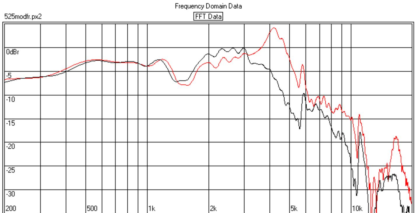
The next example is a transducer with an advertised basket diameter of 4.5 inches and a cone diameter of 3.188 inches, and featuring a stiff paper dust cap. The transducer is claimed full range and the stock performance impulse response and frequency response are shown in figures nineteen and twenty. This transducer has a paper cone body with treated cloth surround and features a small rigid paper dust cap attached directly to the voice coil former.
