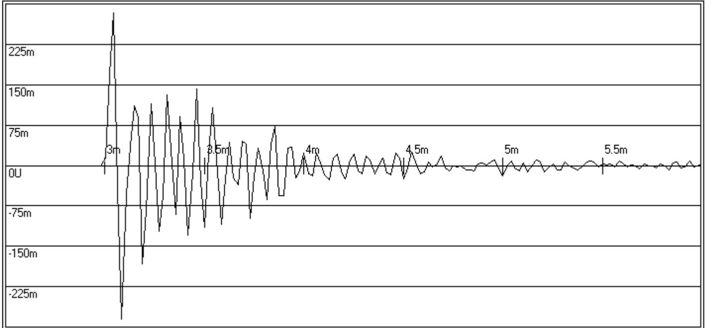
**Figure Twenty. Stock frequency response of paper cone body and dust cap 4.5-inch diameter transducer.**
