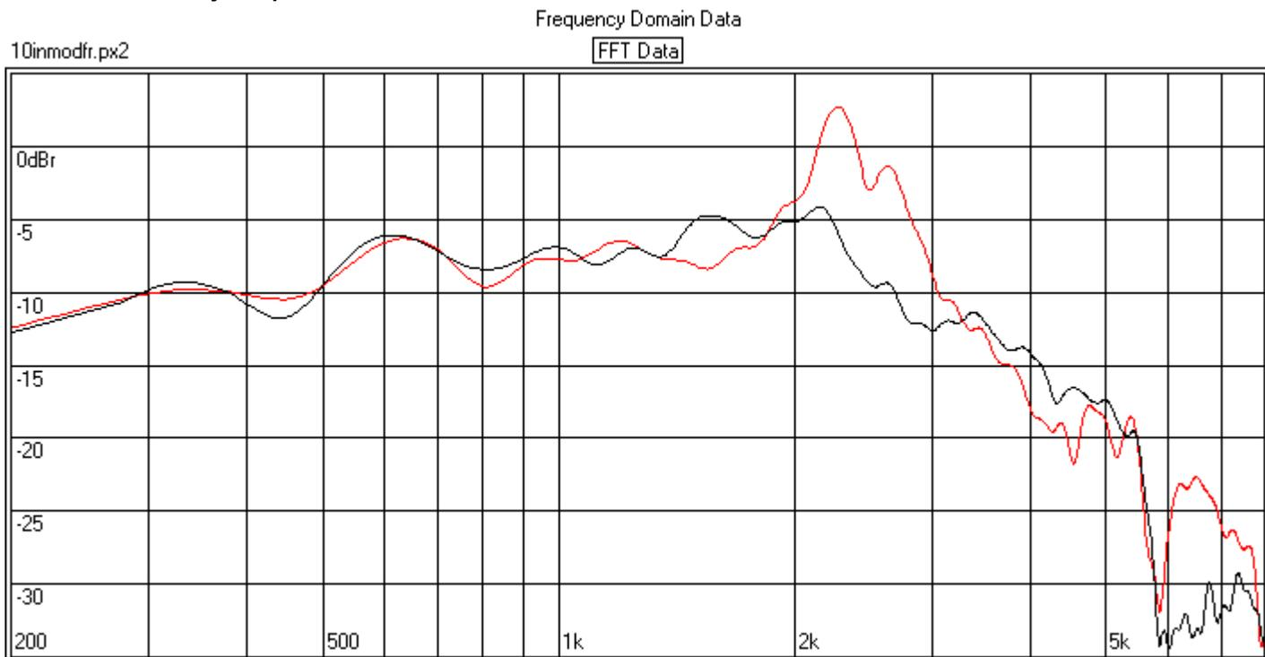
My purpose in including multiple examples in this document in addition to the examples in the patent application is to show that the technique is applicable to all diameter transducers. This second transducer is an advertised eight-inch basket diameter. The cone body and dust cap are made from polypropylene plastic. The voice coil inductance is low and the bandwidth is wider than most eight-inch transducers. This wide frequency response clearly shows how complex vibration modes can become.
