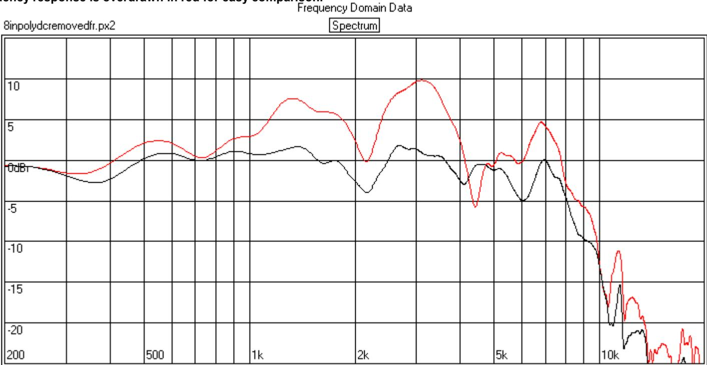
Figures nine and ten show the impulse and frequency response with the dust cap replaced with a plug and the cone dimpled. Only a tiny area of the cone needs to be treated to achieve this quality of performance.
