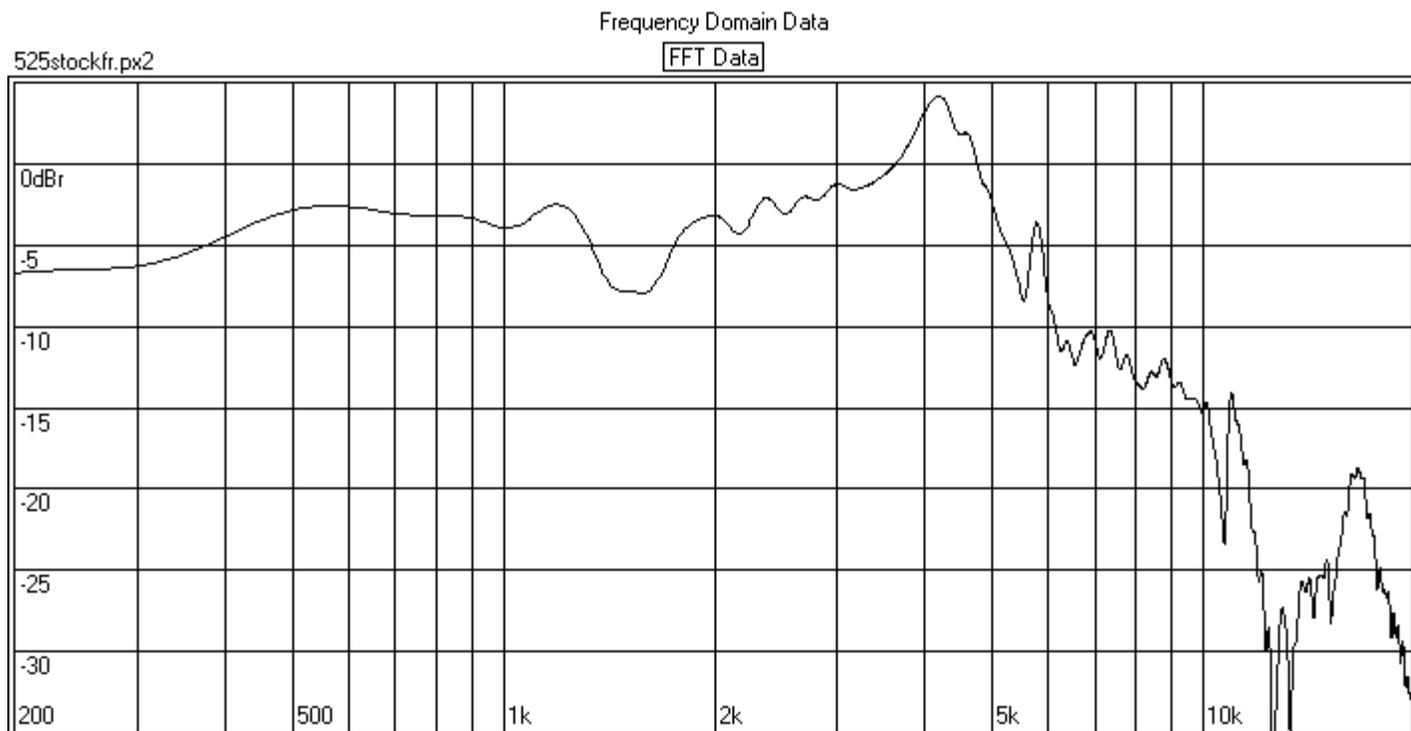
For this relatively soft pulp paper cone, four radial, rectangular shaped dimples effectively controlled the major cone vibration mode. The dimples are 3 mm wide and 10 mm long. Each begins 9 mm in from cone OD.
