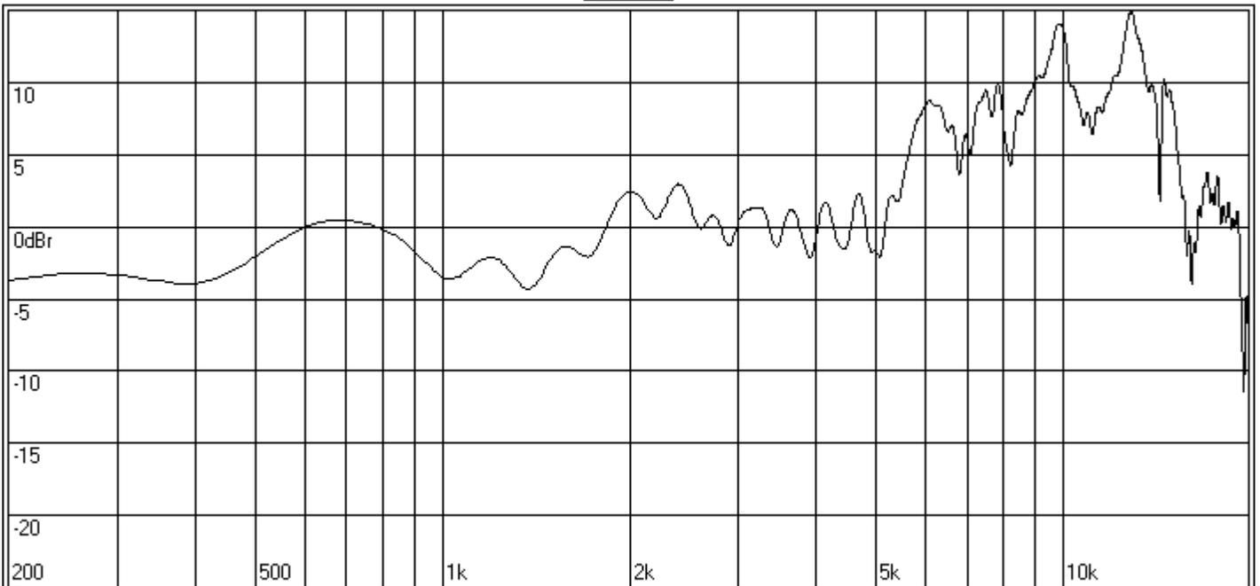
For this example, both the cone body and the dust cap are dimpled. The vibration modes in this example were very complex and produced response problems of great complexity requiring more complex dimpling. The dimpling to the paper cone consisted of 10 rectangular dimples between three and four mm wide and varying from five to ten mm in length. The dust cap treatment consisted of very narrow dimpled areas only one mm wide and varying from two to six mm in length.
